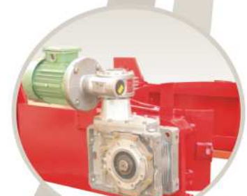
EHDL-50 motorised drum tilting mechanism
